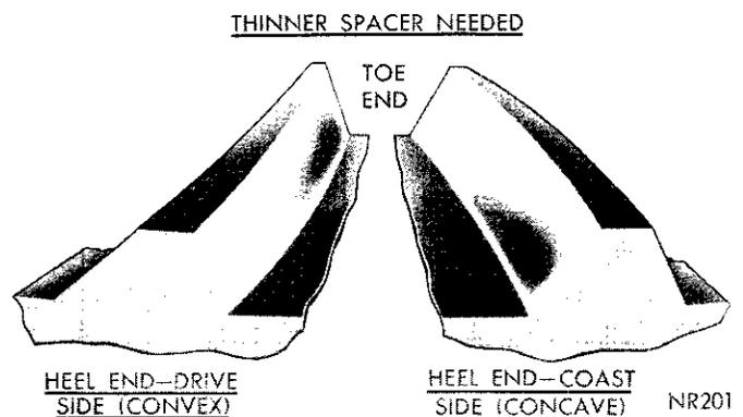
**Fig. 35—Incorrect Tooth Contact Pattern
