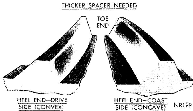
**Fig. 33—Incorrect Tooth Contact Pattern
